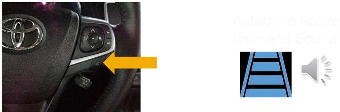
**Figure 2.2 - Autodrive button and instrument cluster icon**
